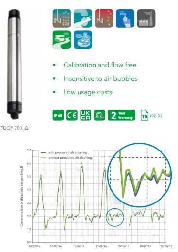
Comparison of two FDO® sensors with and without pressured air cleaning
