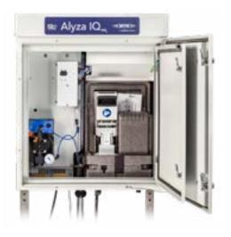
Alyza IQ NH<sub>4</sub> one-channel version with open measuring unit and visible photometer
