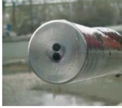
$\mathsf{ViSolid}^{\circledast}$  700 IQ with working ultrasonic cleaning system shows no adverse effect.
